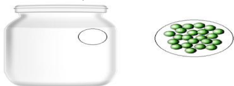
Fig. Irregular arrangement of particles in an amorphous solid
