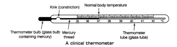
ust above the bulb containing mercury, a clinical thermometer has a kink in its glass tube which is to prevent the back flow of mercury into the thermometer bulb when the thermometer bulb is removed from the mouth of a patient. This kink prevents the mercury level in the thermometer tube from falling on its own. Due to this, we can read the correct body temperature of the patient even after removing the thermometer bulb from his mouth.
